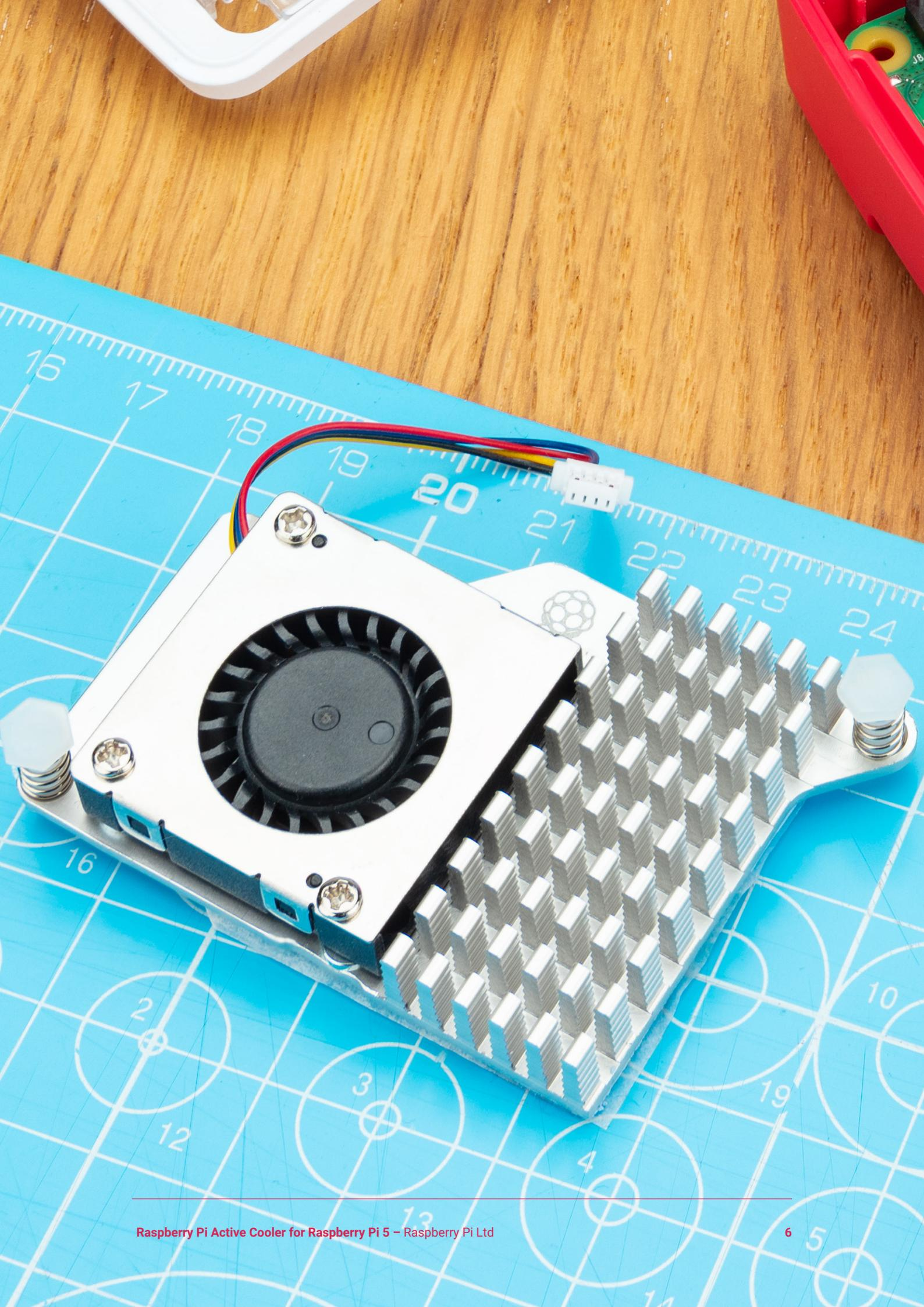
Raspberry Pi Active Cooler for Raspberry Pi 5 – Raspberry Pi Ltd
